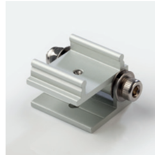
KKBK-21 Adjustable bracket (allow 2 per metre/40in) Anodised aluminium finish L34/W25/H41.9mm (L1.34/W0.98/H1.65") Pre-assembled in factory
